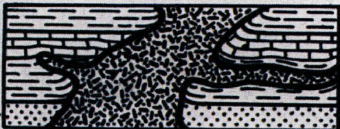
5. IGNEOUS INTRUSION. Sometimes masses of molten rock from deep down in the earth have ascended into the overlying sedimentary rocks perhaps melting their way through and absorbing more or less the materials encountered, and have then solidified.
