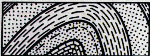
3. ANTICLINAL STRUCTURE. In some cases the beds are found to be bent into an arch-like form called an anticline.
