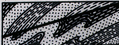
10. FAULTING (THRUST) Faults may also be caused by a push which results in a forward and upward movement of the rocks instead of the normal downward slip and the term thrust is applied to them. This type is most frequent and important in mountain regions.
