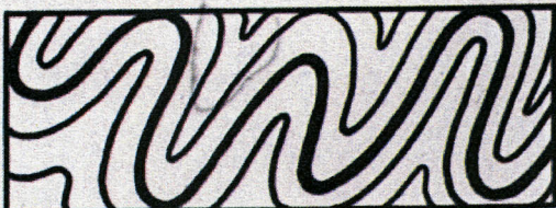
8. FOLDING. When compressional forces are existent the rocks become folded into a series of arches and troughs.
